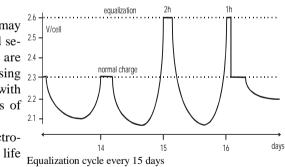
fifteen days a gassing cycle. For about three hours the final charge voltage will be increased to 2.6V/cell. The resulting gassing phase will be finished after three hours of gassing charge (>2.4V/cell). (See figure)
